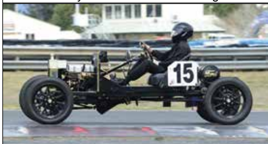
Side-on view of Kevyn Brown's Model T shows the the cylinder head is not the original.
