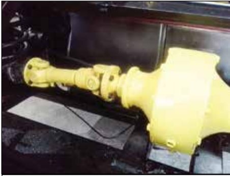
The modified Ford differential with the half shaft running to the trailing arm mounted hub
