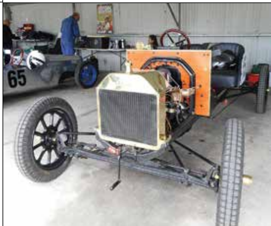
Kevyn Brown's 1915 brass radiator Ford Model T special. That looks suspiciously like an overhead valve conversion rocker cover peeking out from behind the radiator.
