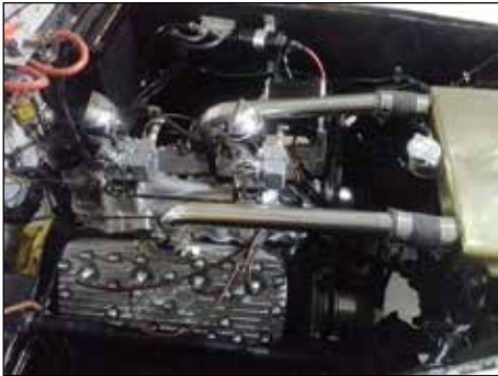
Clockwise from left: The V8 engine with Edelbrock heads; Engine bay showing steering and front suspension; Head on shot showing the grill, headlights and parking lights during restoration; Right front during restoration. Photos on this page from Rodney Williams.
