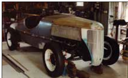
Cranston V8 replica under construction by Max Gamble and Clem Dwyer, both of whom drove it in VSCC events.
