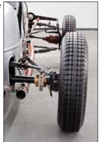
The independent suspension of the Chamberlain Special
