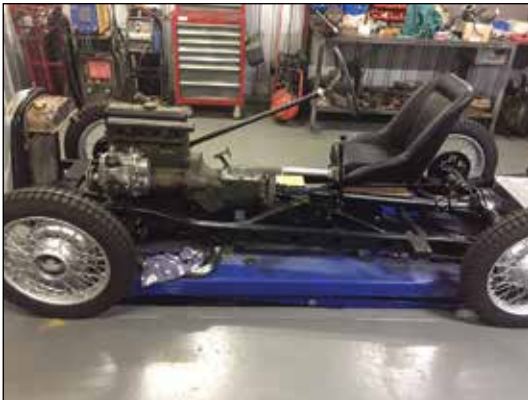
The bare chassis with the blower partly installed
