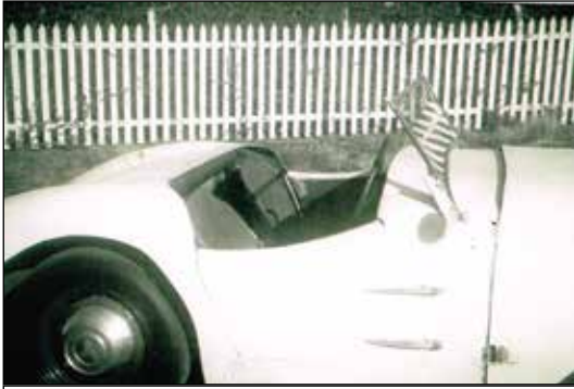
The Stinson car showing the door cut out of the driver's side and the rough fit of the lift up front that replaced the original bonnet opening.
