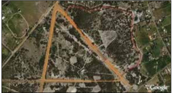
Google Earth view taken in 2012 showing Caversham airfield and its runways, now no longer surfaced, see also visible disused antenna array areas (ground zero), and aircraft dispersal road (D-circuit)
