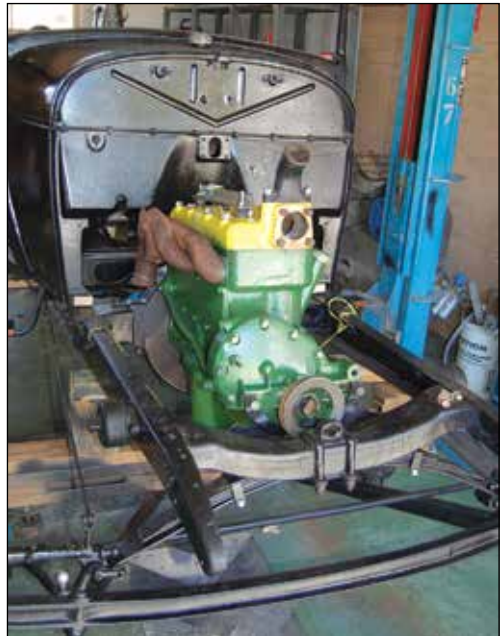
▲ The engine being test fitted in the chassis. ◀ Denny painting the scuttle and windscreen frame.
