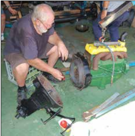
Kevin busy wiring the flywheel bolts. The gearbox sits by his right foot ready to fit.
