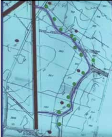
▲ Diagram showing main runway and aircraft taxi and dispersal road. Note: aircraft staging points (green) and machine gun posts (black)
