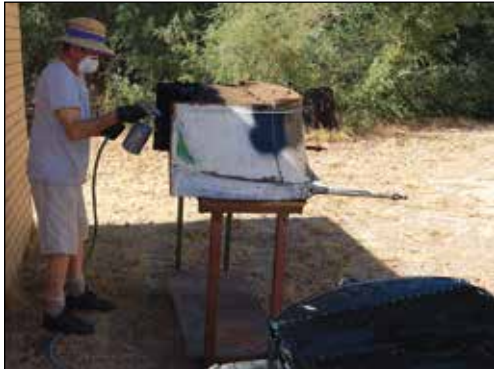
▲ The engine being test fitted in the chassis. ◀ Denny painting the scuttle and windscreen frame.
