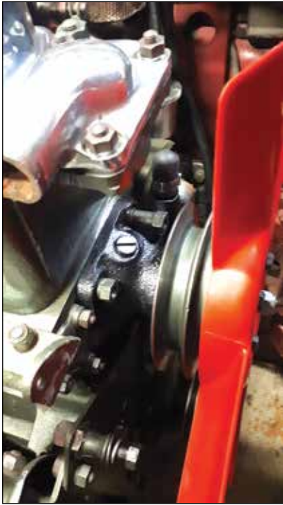
Above: The new water pump installed (and painted black as I'd run out of the correct engine paint)
