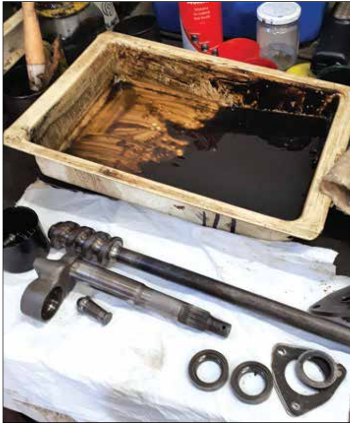
Above: The steering box internals laid bare and the tray of goo drained from the box.
