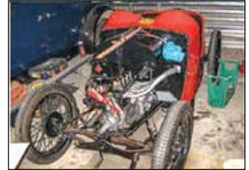
The engine installed with the unique exhaust manifold
