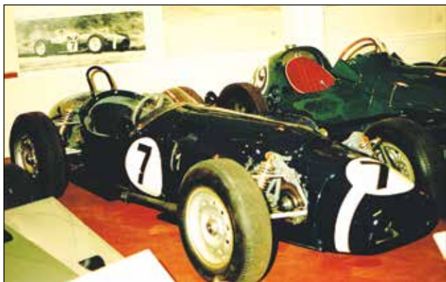
Ferguson P99 at Donington. Last front-engined car to win an F1 race, only 4WD car to win an F1 race. It's different.
