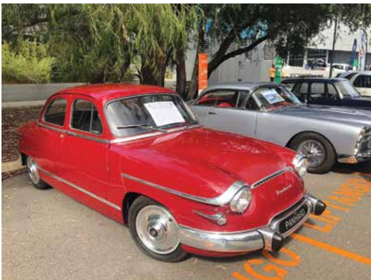
Left: Panhard Dyna with 850 cc and front wheel drive. 80 mph cruising with six people on board was possible because of excellent aerodynamics. Right: two Maserati V6 engine Citroën SM coupés.
