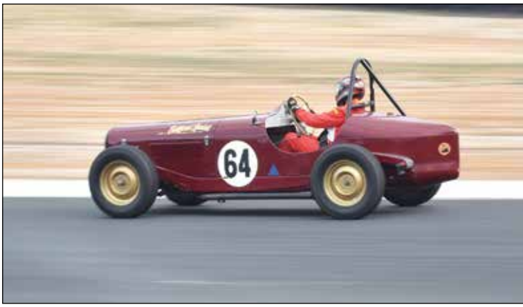
Warwick Milner, Belford Special speeds past the pit exit. The more observant among you will have noticed that the Belford Special does not have a Ford chassis. It is based on a Plymouth chassis with all Plymouth running gear except the engine and gearbox, which are from a Ford V8.
