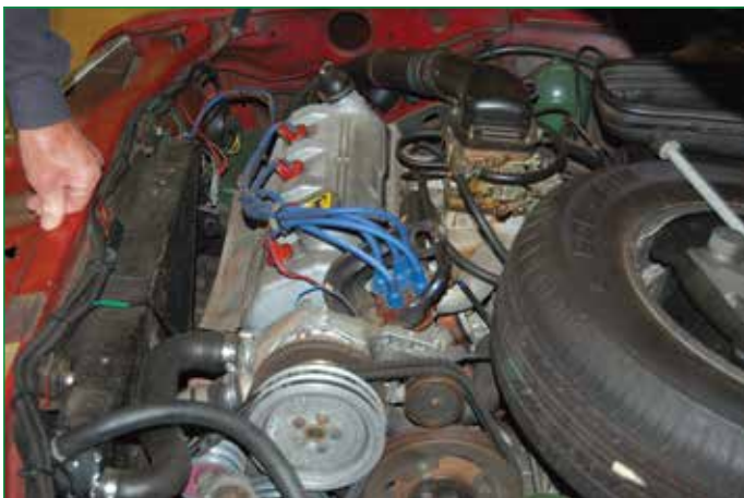
The Citroën engine is tilted forward to lower the bonnet line, but there is still space for the spare wheel in the engine bay.
