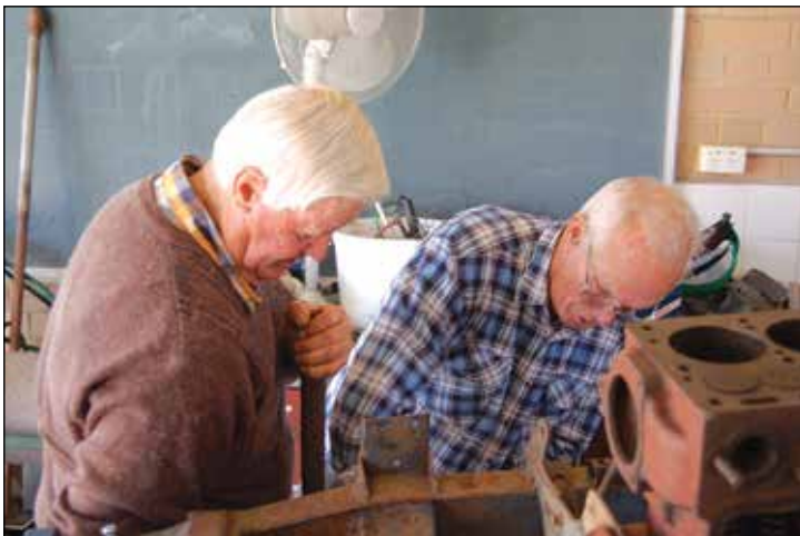
Barry Mackintosh and Robbie Rhodes removing suspension bushes from the Standard chassis.
