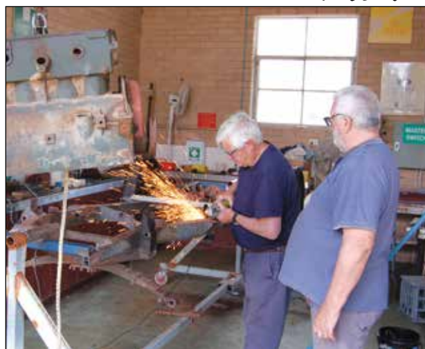
Ian Fry applies the angle grinder to the removal of the gearbox crossmember while Glynn looks on ready to take over.
