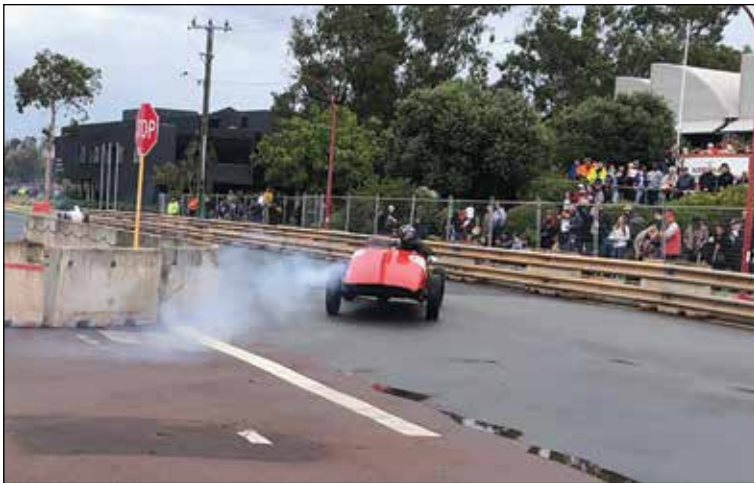
Graeme Cocks smokes his way around in the Ford Cranston V8 courtesy of an overfilled sump.
