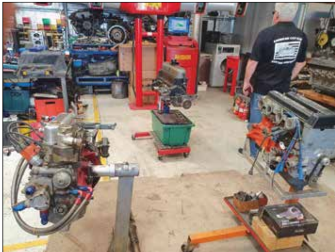
The WARM engine rebuild area with a Ford Formula Junior engine at left, a Lotus Ford twincam to the right and a Holden six behind the green plastic box. MB
