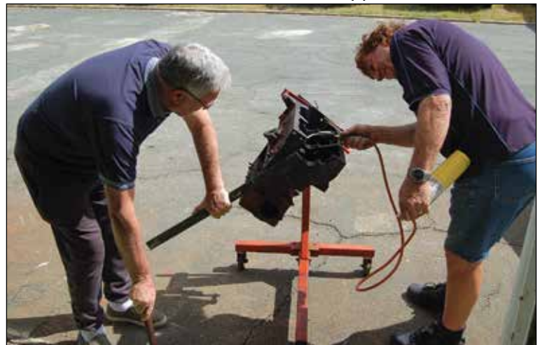
Brian Eyre (left) and Wally Phoebe work on removing the valve springs and valves.
