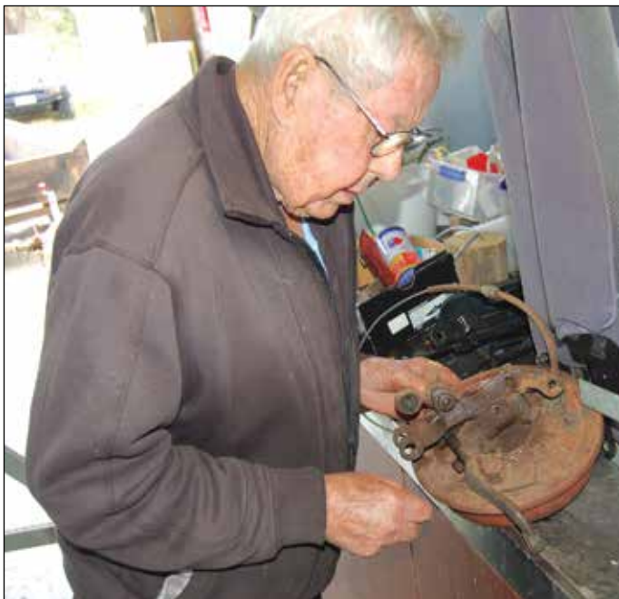
Peter van der Struyf working on a front upright and hub from the Standard chassis.
