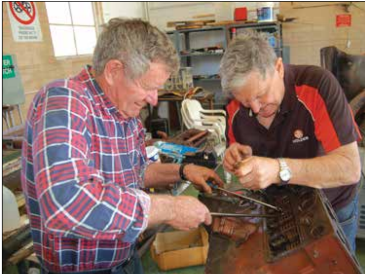
Brian Eyre (left) and Wally Phoebe work on removing the valve springs and valves.
