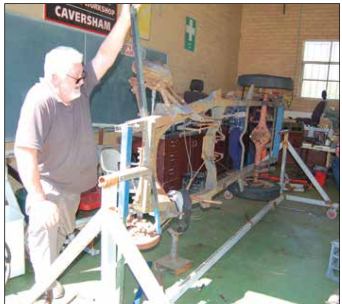
Glynn Allison checks to see that the Standard chassis swings nicely on the rotisserie.
