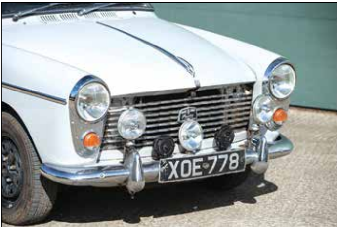
Auxiliary lights and twin horns adorn the front of the A40. All serve a useful purpose.
