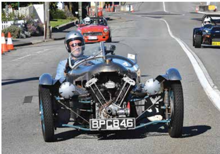
Mike Ognenis, Morgan 3 Wheeler, at the top of Aberdeen Street, Albany in June 2019. Note the JAP V-twin and sliding pillar front suspension, not a wishbone or pull-rod to be seen. Nicole Lothe photograph.
