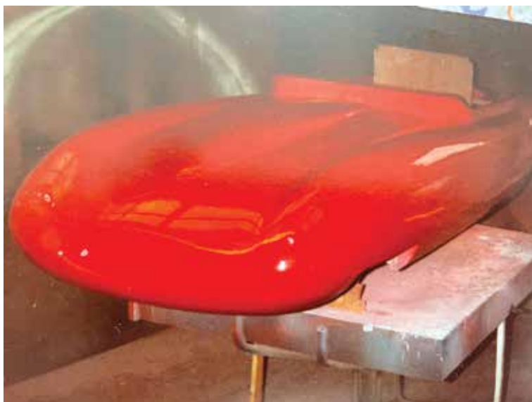
The Elan clay model ready for the moulds to be made.
