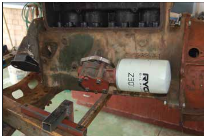
The Holden Red Motor oil pump mounted on the Willys engine using an adaptor as described by Graeme Snape.
