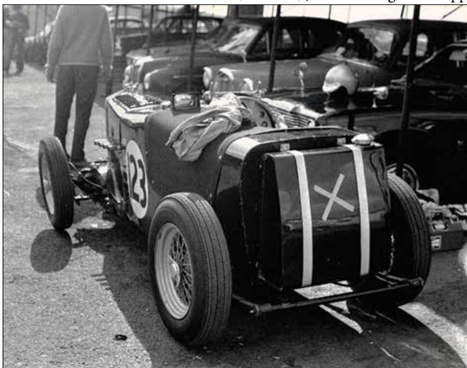
A UK shot of the truncated rear of the lightweight aluminium body as built. Rear wheels are 16-inch with 15-inch rims at the front.
