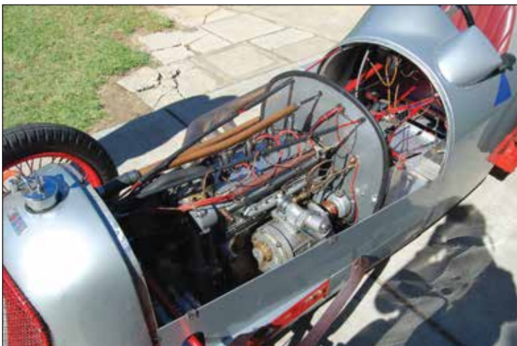
Above: Cockpit view. Note battery box, fire extinguisher and seat belt that Jack Bartlett wouldn't have had.
