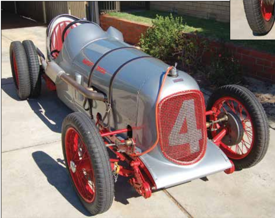
Right front view of the car as it is today. Note the friction shock absorbers and the blow-off pipe for the radiator.
