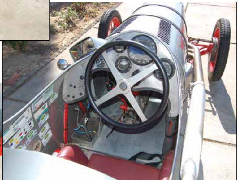
Above: Cockpit view. Note battery box, fire extinguisher and seat belt that Jack Bartlett wouldn't have had.
