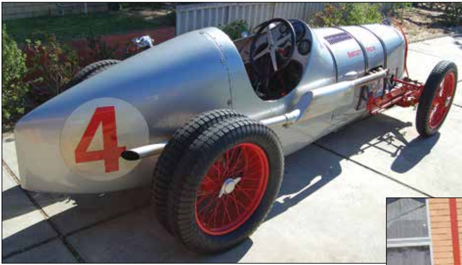
Right rear view of the car as it is today. Note the 'Brooklands' silencer and dual rear wheels as used by Jack Bartlett for hillclimbs.
