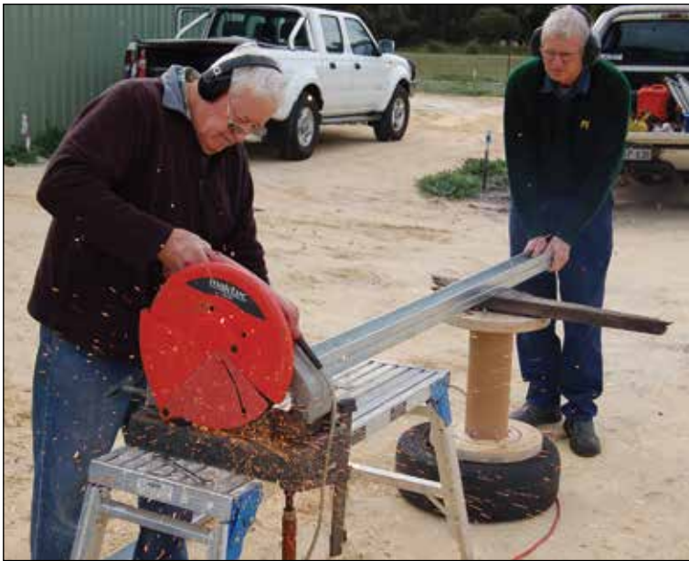
Sparks fly as Barry and Lindsay cut frame pieces to size. Note the high-tech support.
