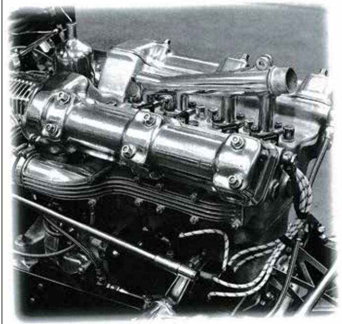
A scan from Karl Ludvigsen's book Classic Racing Engines showing the twin OHC Austin Seven. Ludvigsen said that the only thing it had in common with the production cars was that it had four cylinders.
