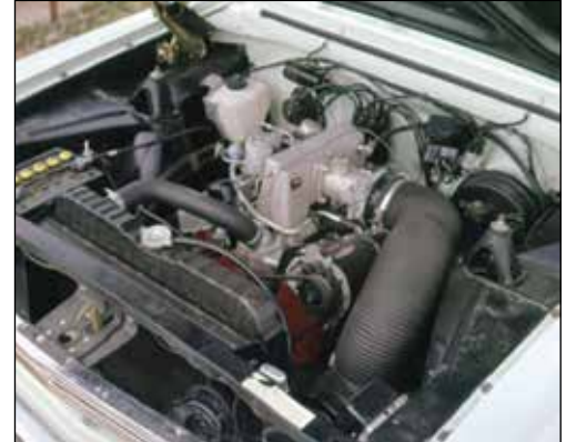
Bill Thomas' very sanitary V8 swap looks OEM. This is the fuel injected engine in the Kelsey car.
